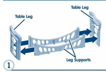
• Fit the leg supports into the slots in each table leg. *Hint:* The leg supports are designed to fit onto the table legs one way. If a leg support does not seem to fit, turn it around and try again!
